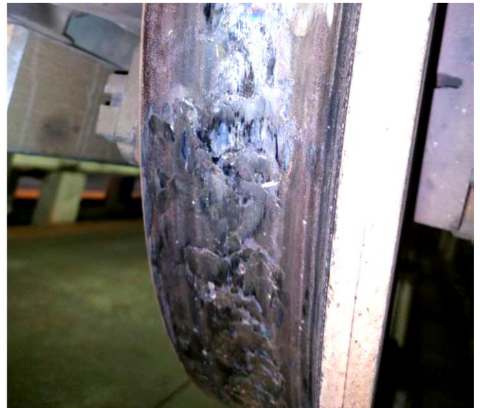
Figure 1. Wheel of TS019 showing extensive damage
