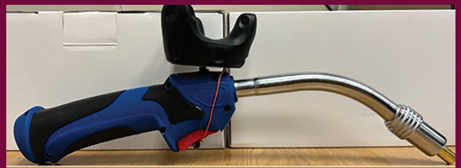
Figure 6: MIG welding torch with tracker.
