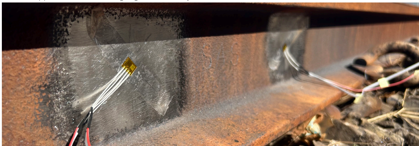
Figure 4: Section of rail instrumented with strain gauges to measure shear strain at the Paarden Eiland depot
