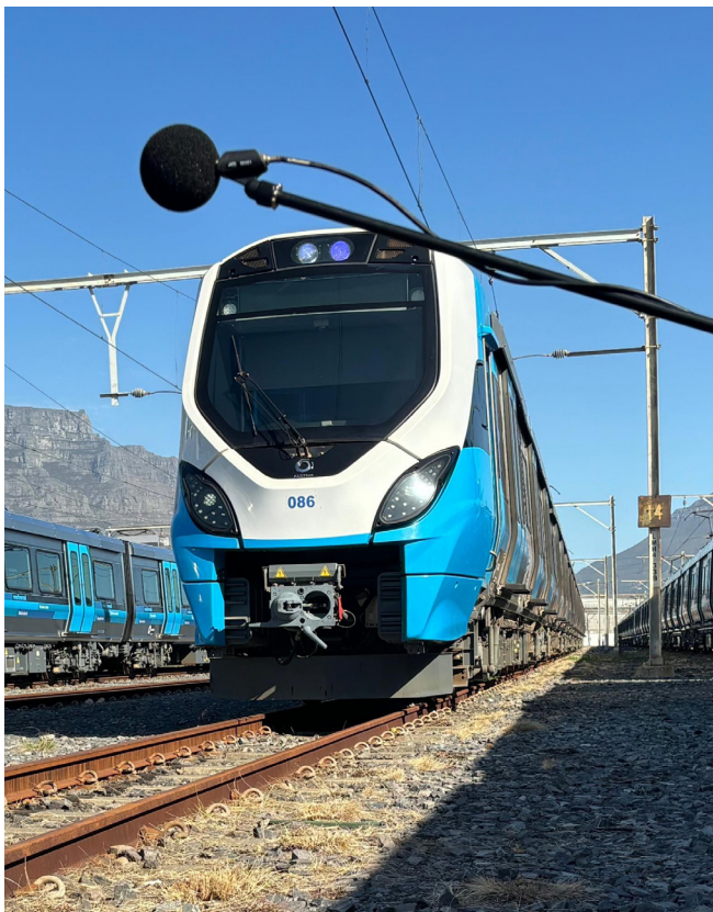
Figure 5: Acoustic sensor used to detect the presence of wheel flats at the Paarden Eiland depot
