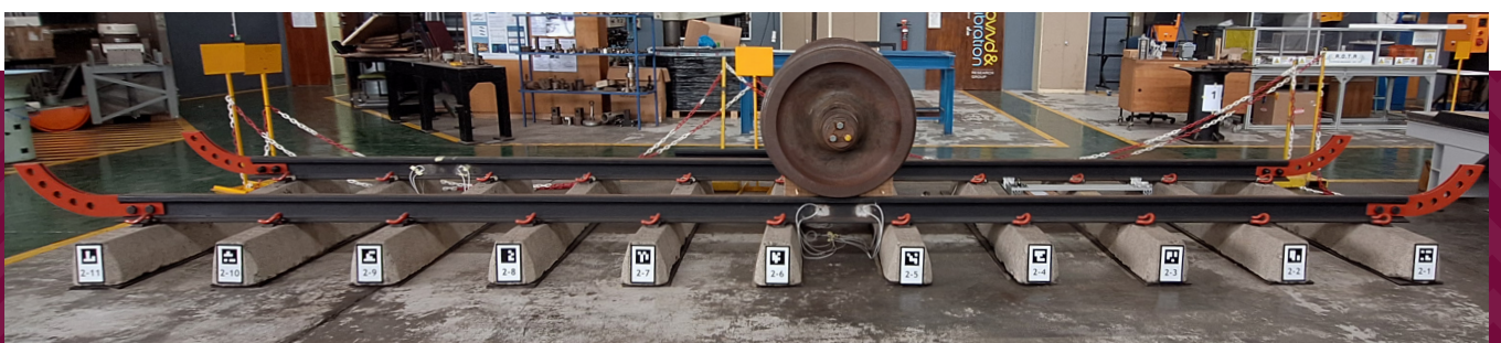
Figure 15: Lateral view of final track laboratory set-up with ArUco markers, single train wheelset and wheel stops
